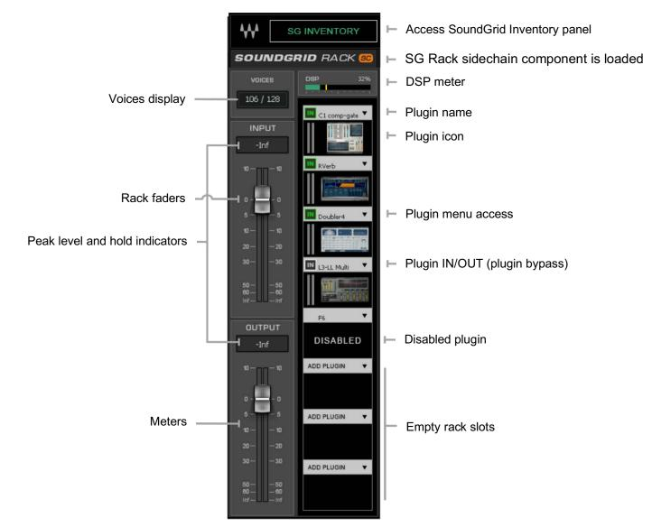
A SoundGrid Rack can be mono or stereo, depending on the status of the channel. Signal flow in a rack is from top to bottom, and if a mono-to-stereo plugin is added to a mono rack, the rack will be stereo from that point on in the signal flow. However, plugins "above" the mono-to-stereo plugin will remain mono.
