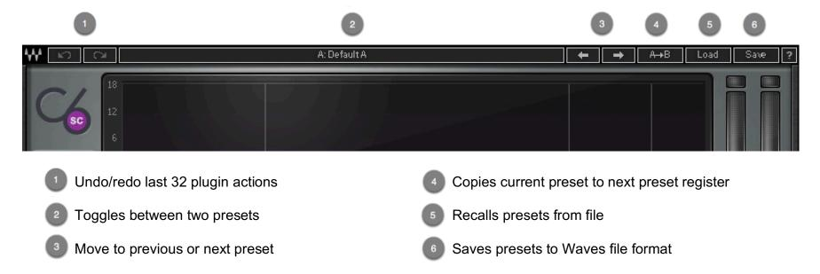
To learn more about the WavesSystem Toolbar and other Waves plugins conventions, refer to the WaveSystem user guide at: www.waves.com/1lib/pdf/plugins/waves-system-guide.pdf
