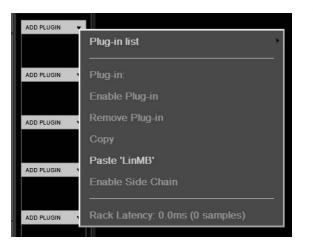
To add a plugin to a SoundGrid Rack, click the arrow on an empty rack slot. This opens the **Plugins Menu**, a multi-level drop-down menu that lists all available plugins. Plugins are organized by category.
