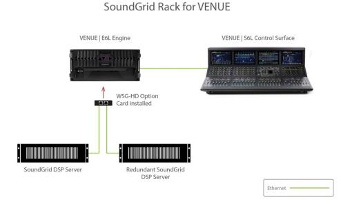
A server can be connected to either port: the physical connection does not determine if a server is the active server or redundant server.
