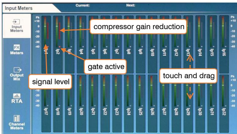
The first three tabs on the **'Meters'** screen show **'Input Meters'**, **'FX Meters'** and **'Output Meters'**.
