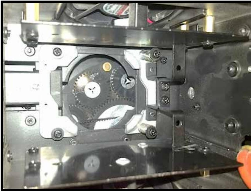
5. Using two fingers on your **RIGHT** hand, pull the retention handle **OUT** and towards the **RIGHT** as far as possible.
