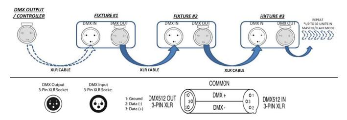
For installations where the DMX cable has to run a long distance, or is in an electrically noisy environment, it is recommended to use a DMX terminator. This helps in preventing corruption of the digital control signal by electrical noise. The DMX terminator is simply an XLR plug with a 120  $\Omega$  resistor connected between pins 2 and 3,which is then plugged into the output XLR socket of the last fixture in the chain. Please see illustrations below.
