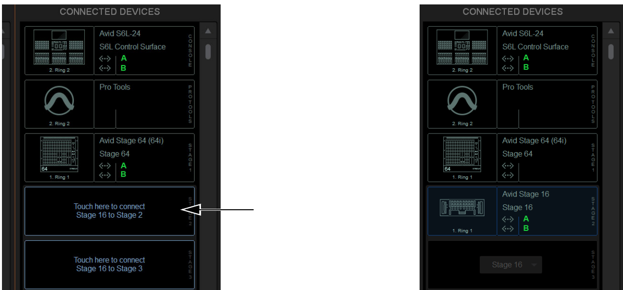
Flashing Stage slots in the Connected Devices column (left) and a Stage 16 assigned to Stage slot 2 (right)
