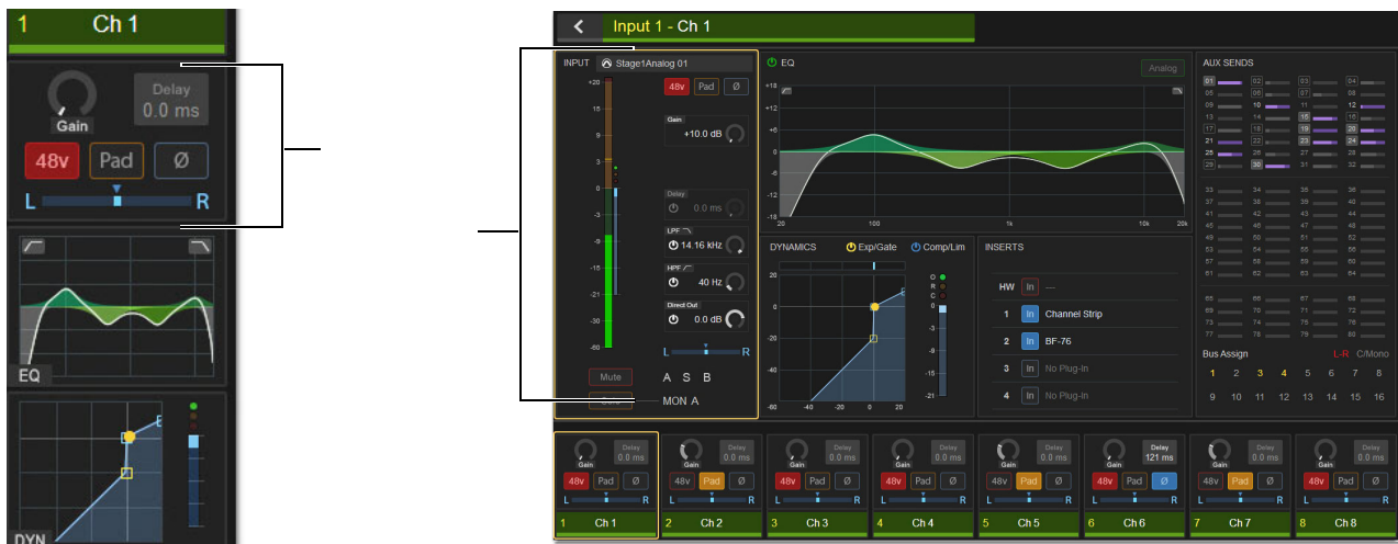
Input touch zone on the CTM in Meters view (left) and in Channel view (right)
