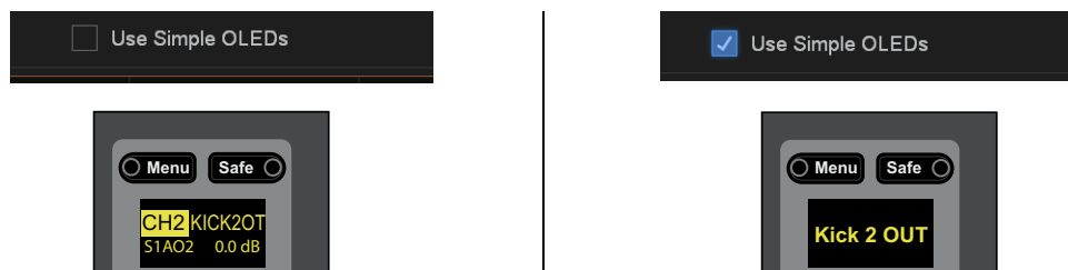
Channel display with Use Simple OLEDs disabled (at left) and enabled (at right)
