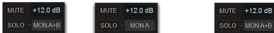
External screen showing a channel routed to Monitor Bus A (Left) Bus B (center) and Buses A and B (right)
