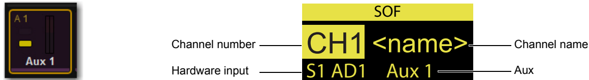
A Channel Tile showing a soloed Aux (left) and a channel display indicating Sends on Faders mode (right)
