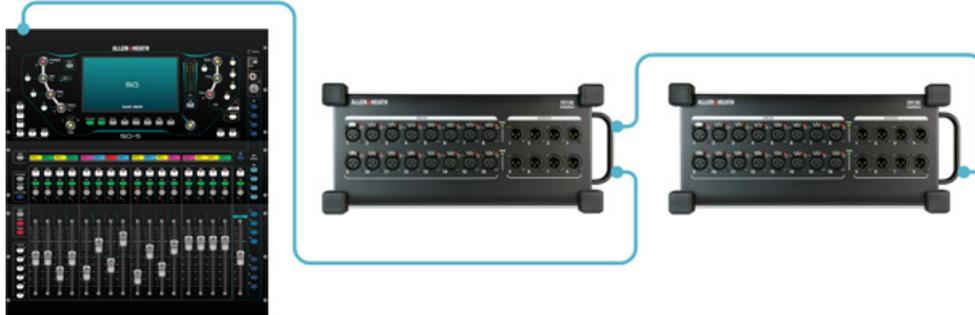
SQ to SQ direct 96kHz connection using gigaACE
