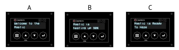
**3.)** Before proceeding, it is important to understand what each button and setting does. Please see the diagram below for button layout. To open settings, hit the menu button, scroll using the Up/Down arrows, and save your setting by pressing enter.
